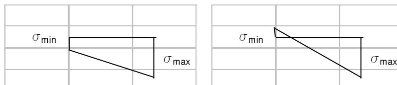
$$p_{\max}(R_x, R_z, B_p, L, h_p, v, P) := \sigma_{\max}(R_x, R_z, B_p, L, h_p, v, P) \cdot B_p$$
