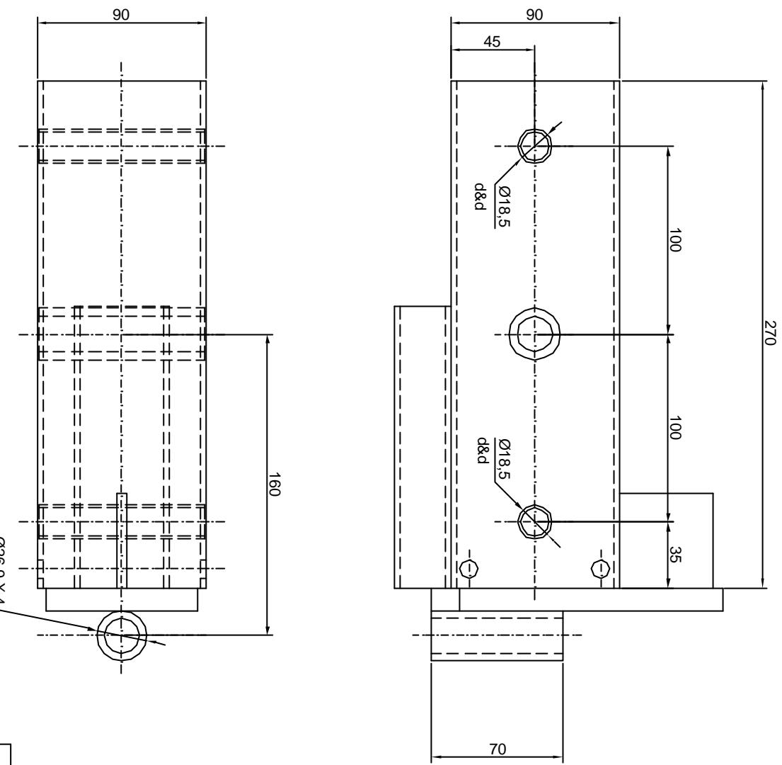
Fig 7: Connection of arch to baseplate
