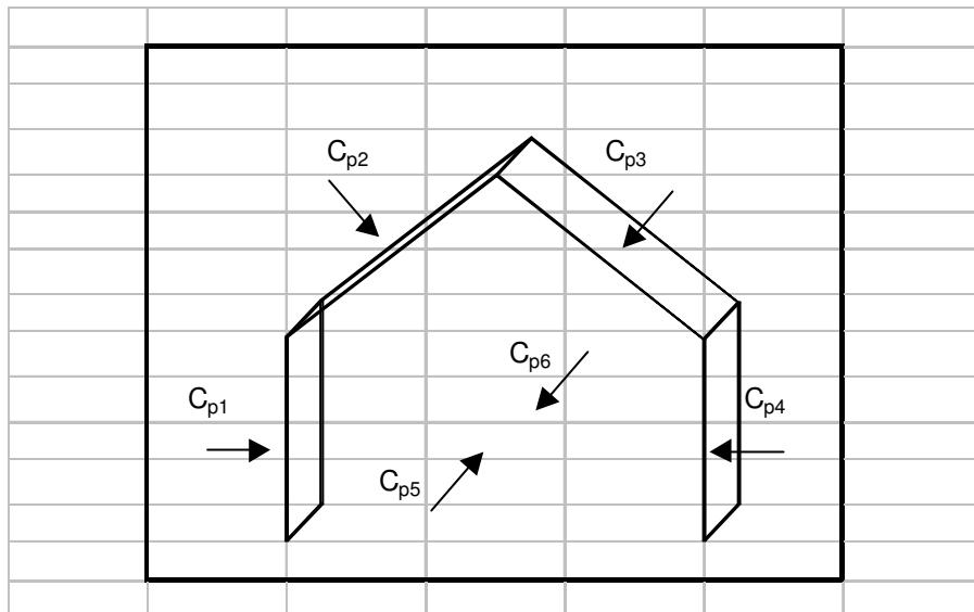
Aerodynamic coefficients for structures of conventional shape (NEN-EN 13782 Fig 2)
