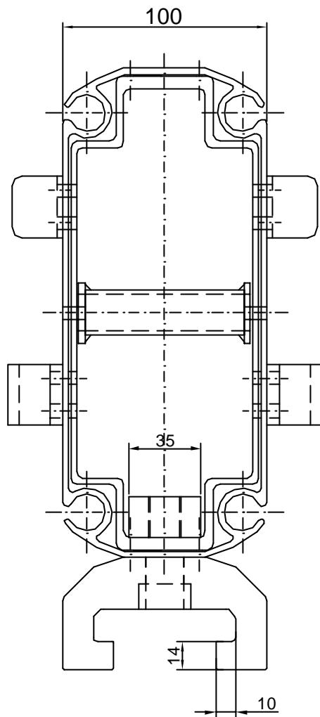
Fig 6: Aluminium rail profile
