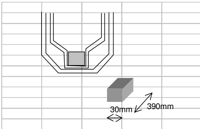
$$F_{pRd} := \frac{(2 \cdot 390\text{mm} + 2 \cdot 30\text{mm}) \cdot t_{alu}(\text{prof\_roof\_prin\_reinf}) \cdot R_{e\_alu}}{\sqrt{3} \gamma_M}$$
