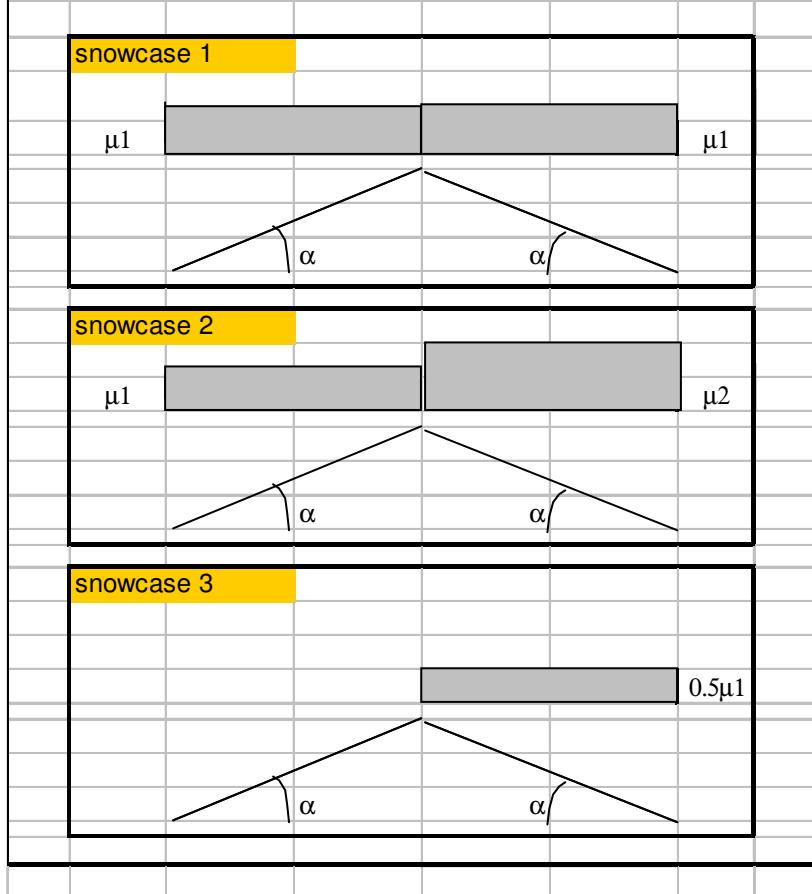
$$\text{snowcase 1 : } s_{1\_windward}(\alpha, p_f, \text{Span\_distance}) := \mu_1(\alpha) \cdot (C_{es} \cdot C_{ts} \cdot s_k(p_f)) \cdot \text{Span\_distance}$$
